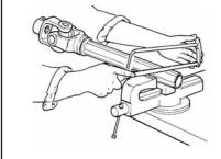
ASSEMBLE THE SHIELDS ON EACH HALF, THEN CUT THE TUBES THE SAME LENGTH AS THE SLIP TUBES. MAKE SURE THEY DO NOT COME TOGHETHER AND BIND WHEN THE 2 HALVES ARE ASSEMBLED.
